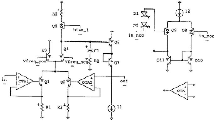
**Figure 1: Bipolar lossy  $g_m$ -C integrator:**
