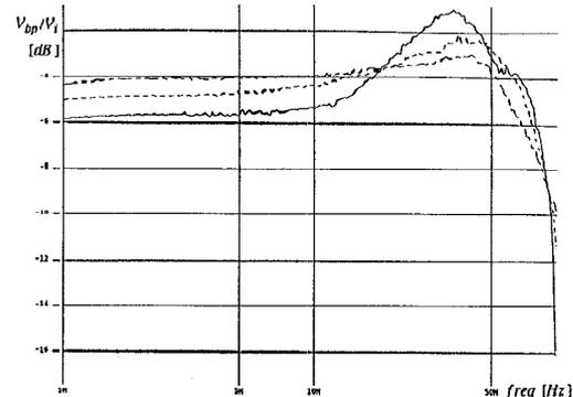
**Figure 6: Measured BP output (3 reference amplitudes and frequency-tuning at 60MHz).**
