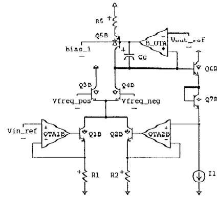
**Figure 2: Bias scheme using the replica of loaded  $G_m$ .**
