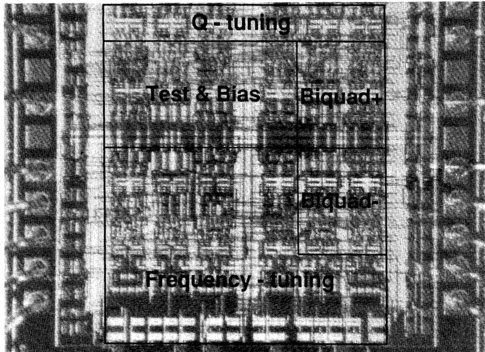
Figure 8: Micrograph of transistor-array filter chip.
