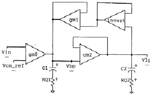
**Figure 3: Single-ended biquad with two lossy integrators.**
